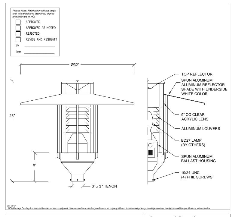
**Diffuser Type:** Acrylic U.V. stabilized clear cylindrical diffuser.
