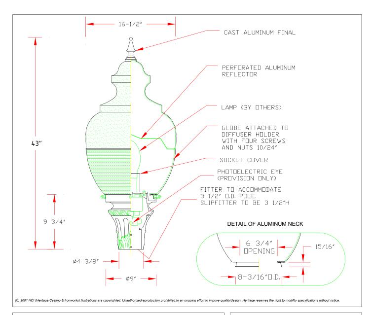
**Diffuser Holder Material:** Cast aluminum. Diffuser is attached with 4 stainless steel screws.
